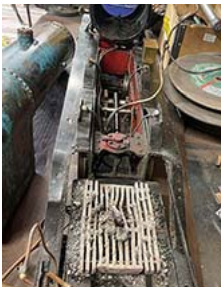
The underframe with the boiler removed. Note the distorted firebars!
