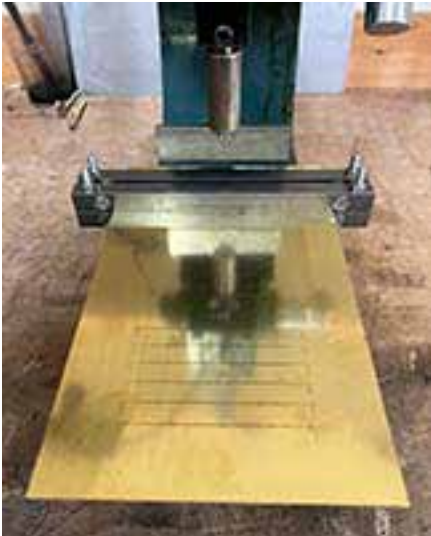
The brass sheet with laser cut slots being placed into the jig. Photo by Maurice Hartnell.
