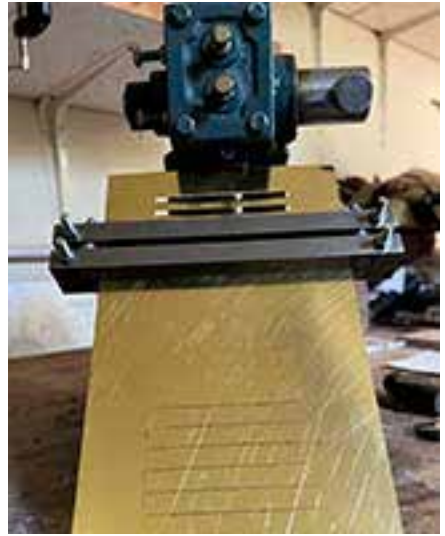
The first two louvers punched out. Photo by Maurice Hartnell.
